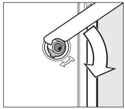
■ Turn the right shipping strut clockwise 90° with the enclosed combination wrench.
